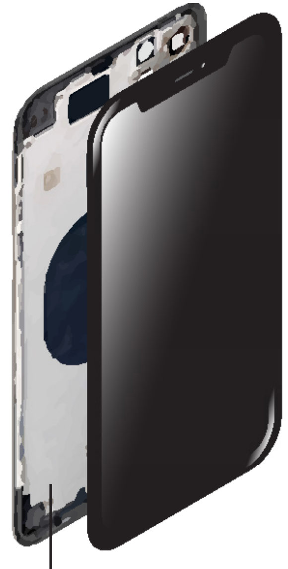
iPhone 11 Pro Chassis (inner structure of the phone model) bound together tightly with strong adhesive glue, to prevent water and dust from passing through.
