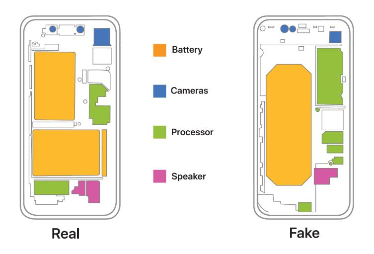
The inside of a fake and real lphone x reveals many differences such as the swap from a dual to standard battery in the fake. The fake's interior parts is also missing the face id sensor and OLED display as it is more expensive to implement.
