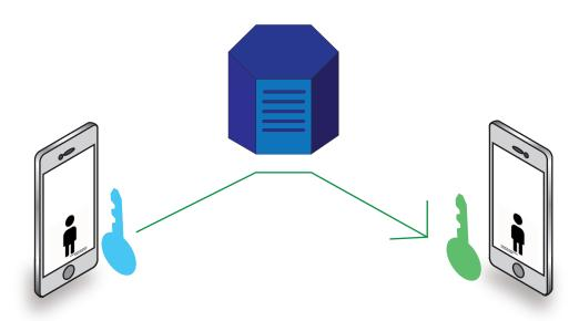
The server is only used to transmit the encrypted message. Only the receiver's private key can unlock the message. No third party including WhatsApp can read the message.
