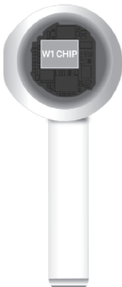
The W1 Chip inside the AirPods
