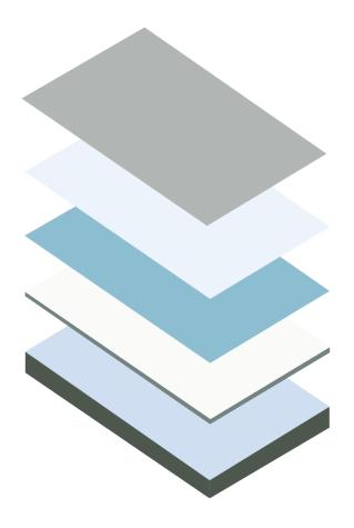
The vast majority of devices that incorporate this touch system utilise censors to monitor and track the finger as it moves around the screen. The iPhone in particular uses electrical currents for a speedy-response time. This is referred to as capacitive touch screens, where a layer of capacitive material holds a small amount of electric charge. This charge is then altered as the user's finger makes contact with the screen.
